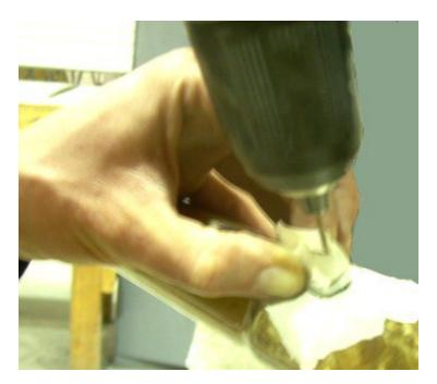
Scrape away the clearcoat and sand the area to be glued. Apply epoxy glue (fine sanding dust and epoxy) to frame and stick cable guide on using the screw as a locator. Screw the cable stop down. If the cable stop does not sit perfectly on the frame, allow the glue to form a base for it. You may not want to screw it down very tight in order to allow the cable stop to be in the best position. Wipe off excess glue as neatly as possible. Let glue harden, then remove the masking tape.
