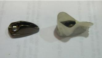
Using the cable stop as a guide, hold the cable stop in position on the wrapping and start drilling the pilot hole. Take away the cable stop and continue drilling through. The wrapping will prevent the bamboo from splitting near the hole. **Do not drill holes into the bamboo that is not covered with wrapping**.
