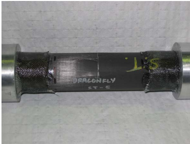
Figure 10. Hy-Bor Seat Tube After Impact Damage
