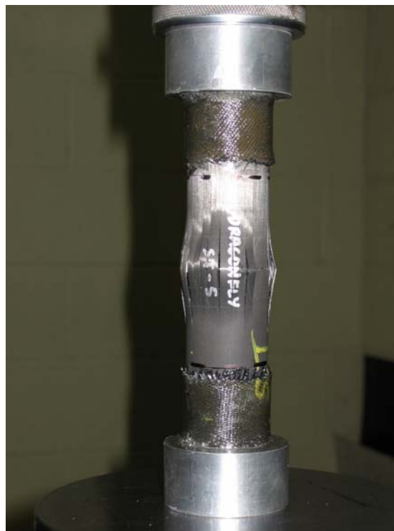
Figure 11. Hy-Bor Seat Tube After Compression Testing
