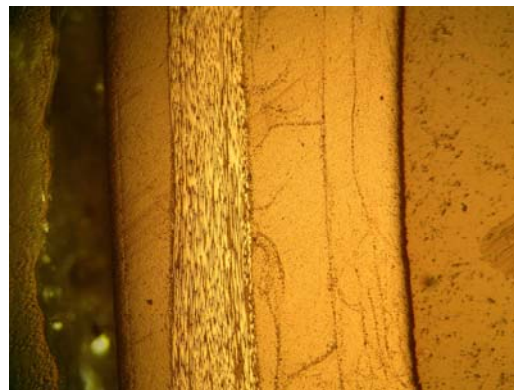
Figure 3. Cross-Sectional View of Graphite/Epoxy Seat Tube
